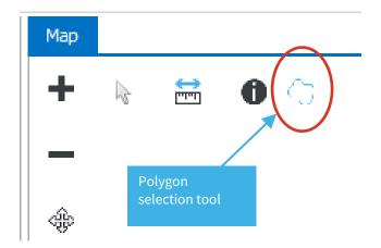
Left click on the map to start drawing your selection polygon. Each subsequent click will add extra points. The polygon will be displayed as a semi-transparent, yellow shape. To end drawing click with the Ctrl key depressed. The nodes within the polygon will be highlighted and the selection mode will be returned to the default mode (i.e. rectangle selection).
