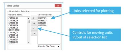
Once the parameter and timing are selected clicking the plot button will generate a chart showing data from all selected units together:
