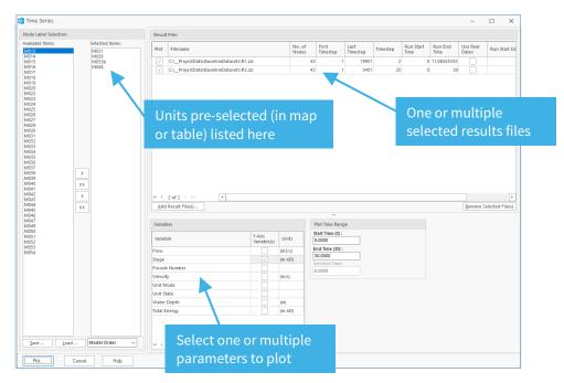
The enhanced plot definition window applies to all 1D plot types, i.e. time series, long sections, cross sections and XY plots.
