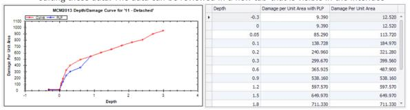
when you select the option to apply property level protection. Furthermore, the impact of a chosen property level protection can be inspected on the damage curve plots, which can show with and without property level protection curves together.
